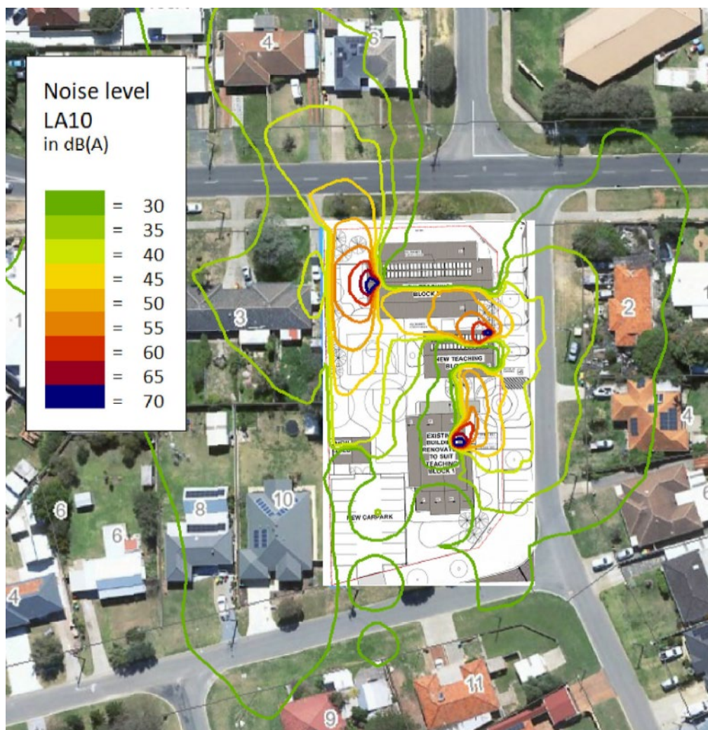
FIGURE 6.7 – NOISE CONTOUR PLOT FOR MECHANICAL SERVICES
