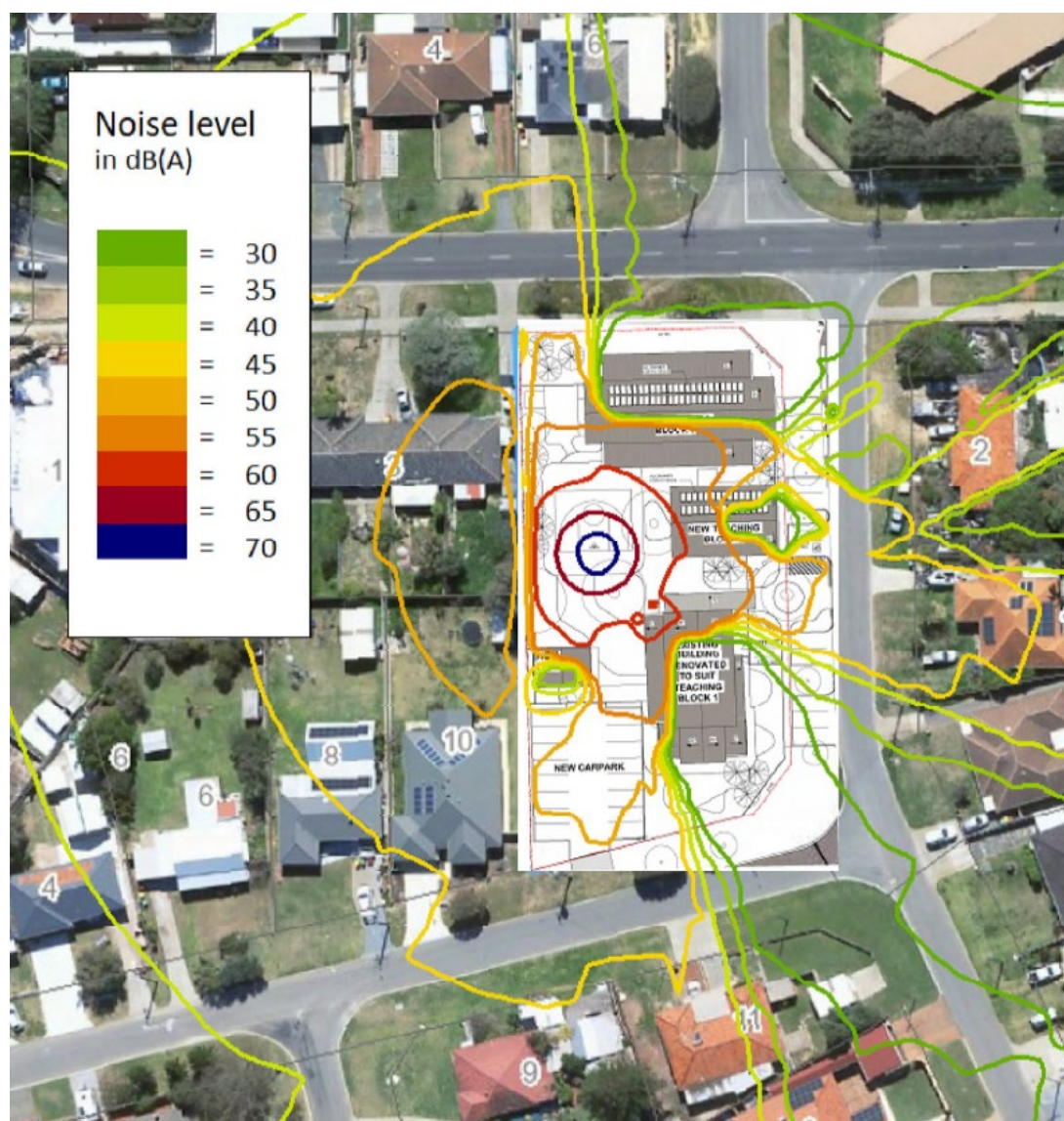
FIGURE 6.5 – NOISE CONTOUR PLOT FOR BASKETBALL HITTING BACKBOARD
