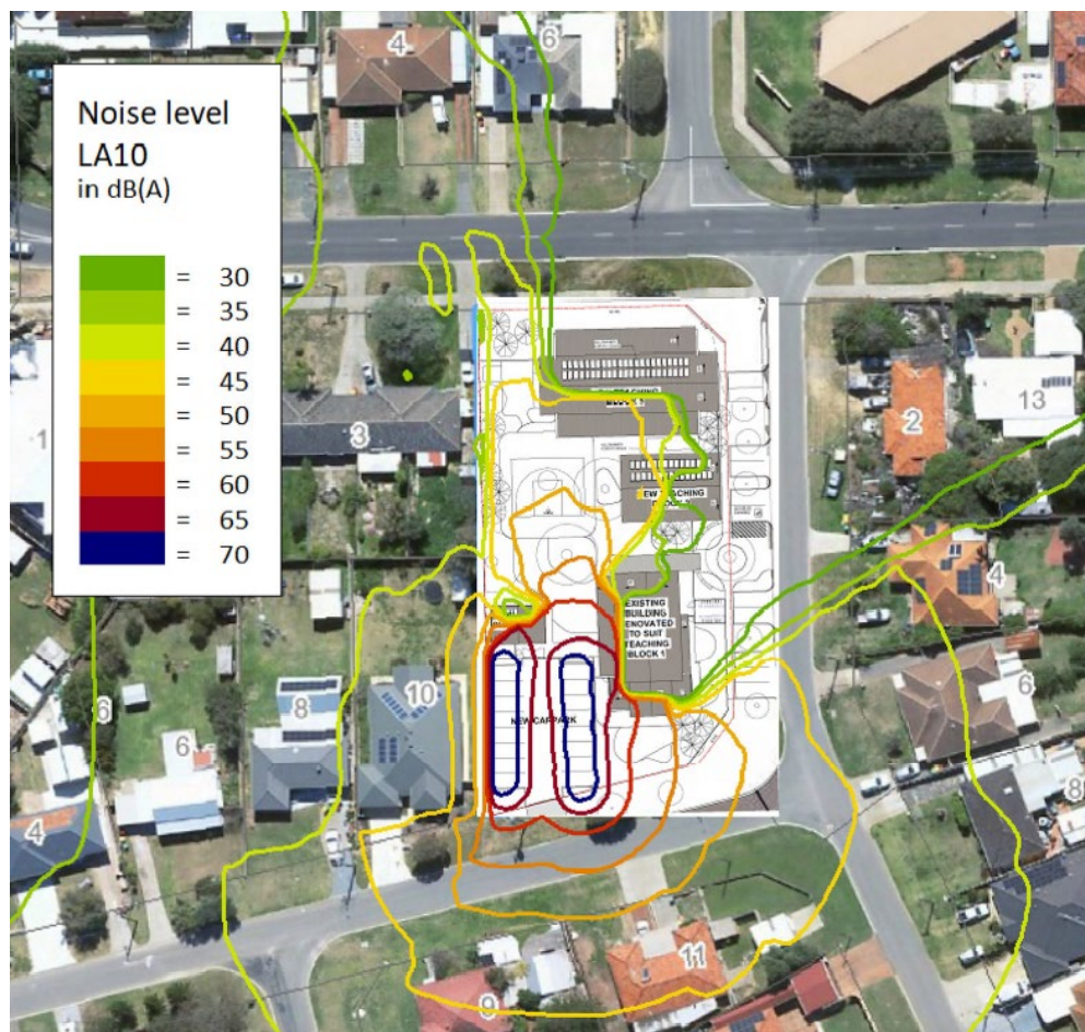
FIGURE 6.8 – NOISE CONTOUR PLOT FOR CAR DOOR
