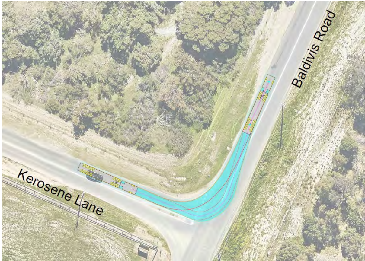
Figure 13 – 19m Semi-trailer Swept Path – Baldvis Road/ Kerosene Lane Intersection – Left turn
